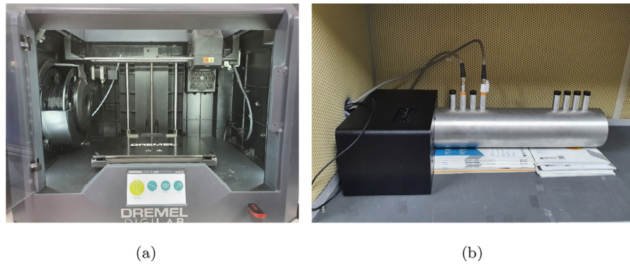
Fig. 1. 3D printer and acoustic experiment setup. (a) 3D printer DREMEL DIGILAB and (b) an acoustic experiment for absorption coefficient (Two points measurement approach, the diameter: 0.1 m, and cutoff frequency: 1929 Hz ([3,20,22,25,26])).
