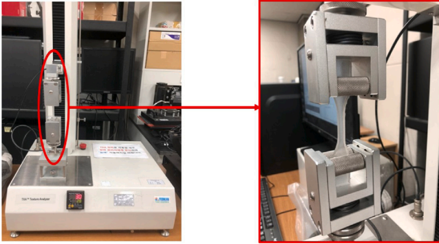
Fig. 4. TXA texture analyzer for tensile test of PDMS specimen.
