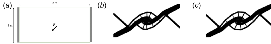
Fig. 17 (a) Design domain and the boundary condition for cantilever box shape, (b) optimum layout for \beta = 0 ( C = 1.7041 J) and (c) \beta = 50 ( C = 1.7774 J)
