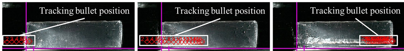
Fig. 4 Projectile position tracking using the captured images and Tracker software
