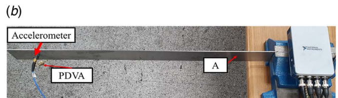
Fig. 10 Experiment 1: the bending vibration of the beam ( L = 0.65 m) (the first-bending mode of the beam: 4.0 Hz, the pendulum frequency: 4.0 Hz, and the spring-mass frequency: 4.0 Hz)
