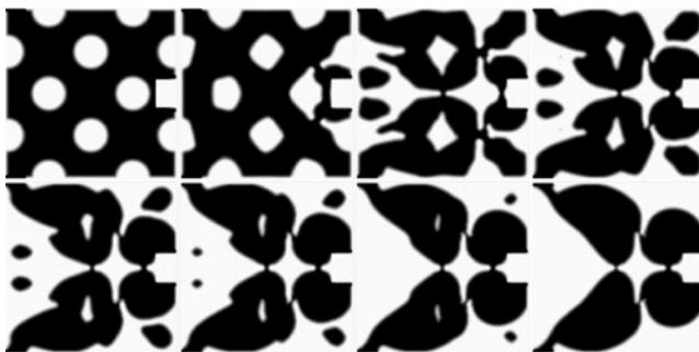
Fig. 16 Plot of the evolving element densities of a compliant gripper design problem using the level-set method combined with ECP
