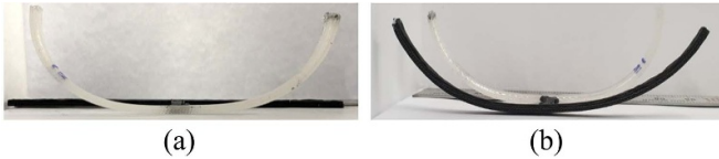
Figure 4. Structural bending of the reference H-beam structure: (a) at 105 °C and (b) at 125 °C.
