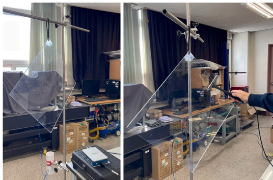
Measures made to satisfy free-free boundary condition
