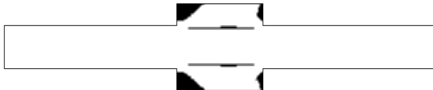
Fig. 8. Optimized membrane layout with the enlarged design domain (optimization procedure termination was due to the numerical errors in the analysis and optimization).
