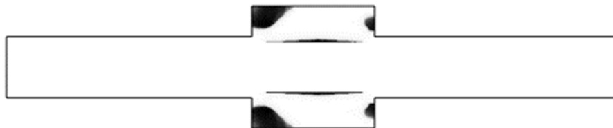
Fig. 9. Optimized design with refined mesh (0.0313 m by 0.0313 m and mesh size = 0.015625 m by 0.015625 m in this RANS model where the Kolmogorov length scale ( \eta = (v^3/\varepsilon)^{1/4} \sim 0.001 m for DNS).
