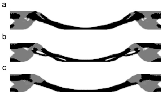
Fig. 9. Optimization results with a homogeneous boundary condition (clamp conditions for both materials). (a) The obtained result with F=2.5 N, (b) with F=5 N, and (c) with F=10 N.
