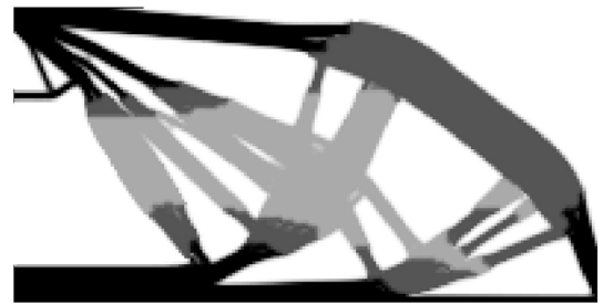
Fig. 17. Topology optimization of MBB with 3 materials, compliance = 0.279 (different colors represent different materials).
